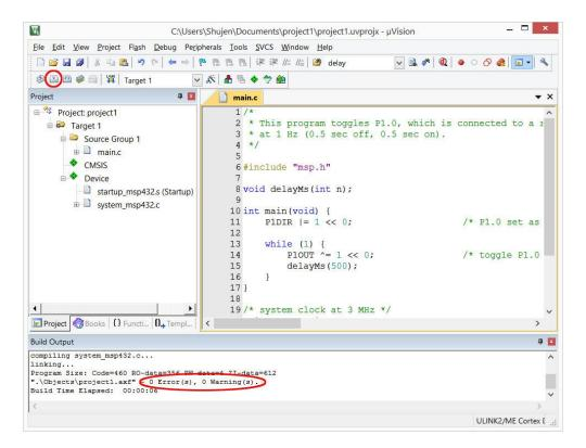
27. Before downloading the program to the target, we need to set up the connection between the uVision IDE and the in-circuit debugger on the target circuit board. Click on the **Target Options** button.
