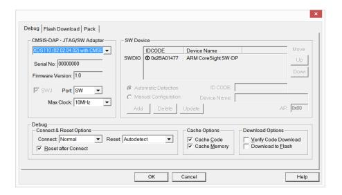
32. To debug the program, click the **Debug** button on the right. The program should automatically download to the target device and the Keil IDE will change the perspective to debug.
