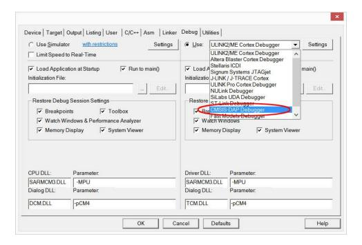
29. Check the box before Load Application at Startup and Run to main() if they are not already checked.
