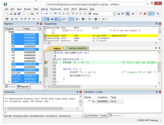
35. The program counter is at the first executable line of the main() function as indicated by the yellow arrows in both source file and disassembly window.
