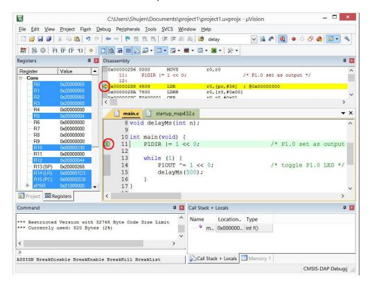
36. Click the **Run** button and the program execution should start. If everything has been done properly, the red LED on the LaunchPad should be blinking.
