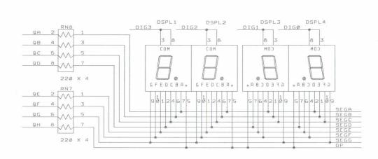
The digit 3, 2, 1, and 0 are driven by QA, QB, QC and QD of the second HCT595, respectively. The 7-segment LED display is turned on one at a time at a high refresh rate. It's fast that our eyes will perceive that all 4 digits are turned on at the same time. To display the number 1234 on the 7-segment display, the following steps should be taken:
