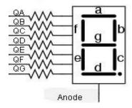
The segment A, B, C, D, E, F, G and Decimal Point are driven by QA, QB, QC,QD,QE, QF,QG, and QH, respectively. The hex value of the segment code is shown in the following table:
