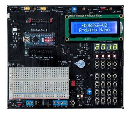
The board will switch VCC from 3V to 5V automatically when a Arduino Nano is plugged in.
