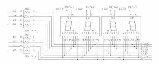
The digit 3, 2, 1, and 0 are driven by QA, QB, QC and QD of the second HCT595, respectively. The 7-segment LED display is turned on one at a time at a high refresh rate. It's fast that our eyes will perceive that all 4 digits are turned on at the same time. To display the number 1234 on the 7-segment display, the following steps should be taken:
