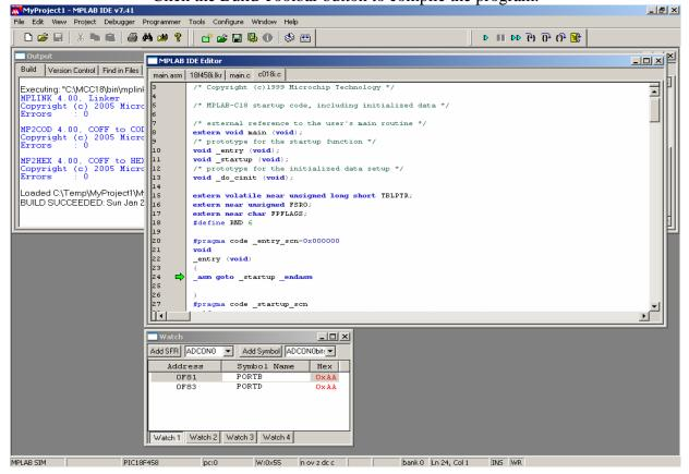
To simulate the program, set a breakpoint by right-clicking the line and selecting Set Breakpoint.
