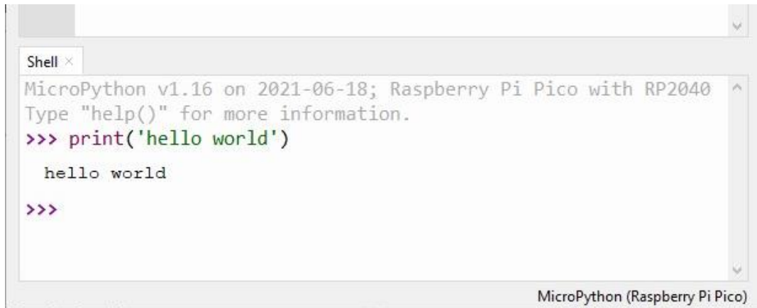
Figure 1-15: The REPL prompt in the Shell pane works the same except the outputs have different fonts and colors for different contexts.
